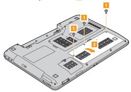
Remove the frame fixing screw.
